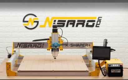
X Shaper Cut MDF, Hard/Soft Wood, Acrylic, Foam, HDPE & other type of plastics & Aluminium etc.
